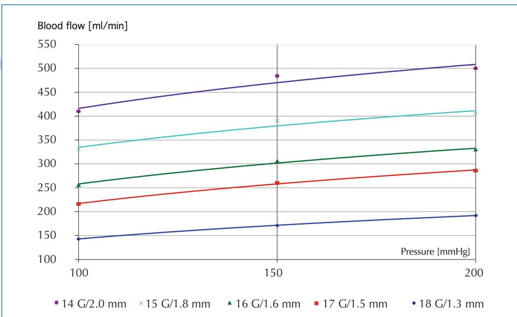
Low flow resistance is a special feature of Bionic Fistula Needles. Extracorporeal blood flows of up to 350 ml / min are within the range of standard 15 G (1.8 mm) needles. For blood flows of 250 ml/min, 16 G (1.6 mm) needles are recommended.
