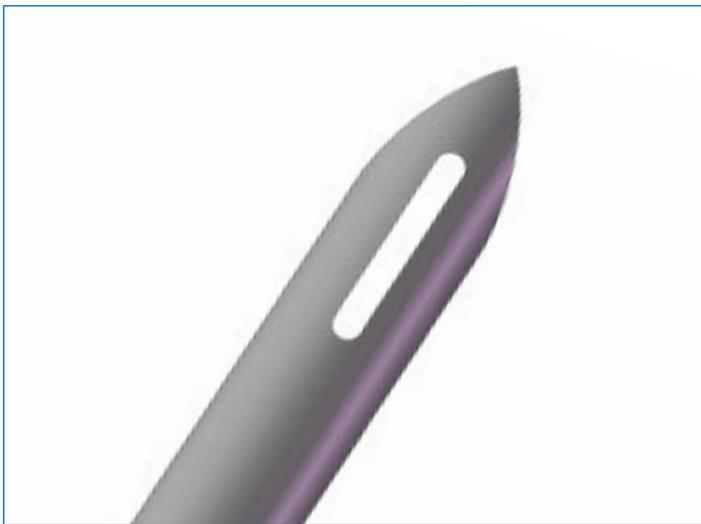
The slit-shaped back eye invented by Bionic is cut from the outer to the inner surface and afterwards rounded accurately. The specially shaped back eye prevents lesions of the vessel's inner surface and assures high blood flow without blockage of the needle.
